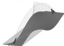
Mode 5 ( f_5 = 1.09\text{Hz} ) Torsional
