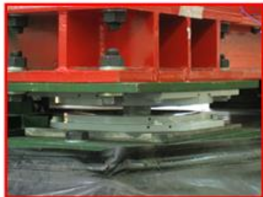
sliding pendulum bearing
