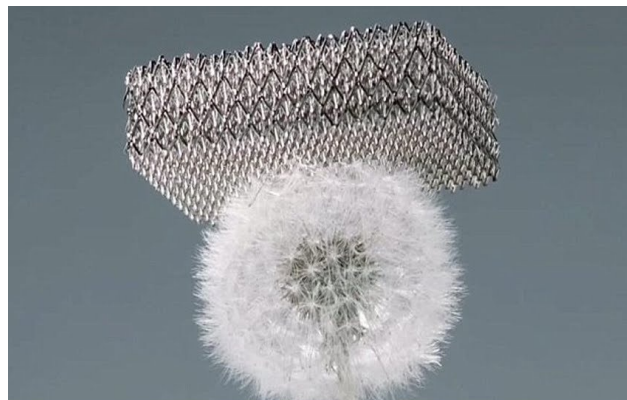
Micro lattice, produced via Additive Manufacturing (Boeing)
